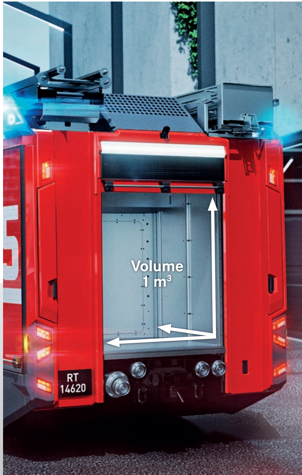
Additional equipment space is available in the rear thanks to the pump unit being moved forward.
